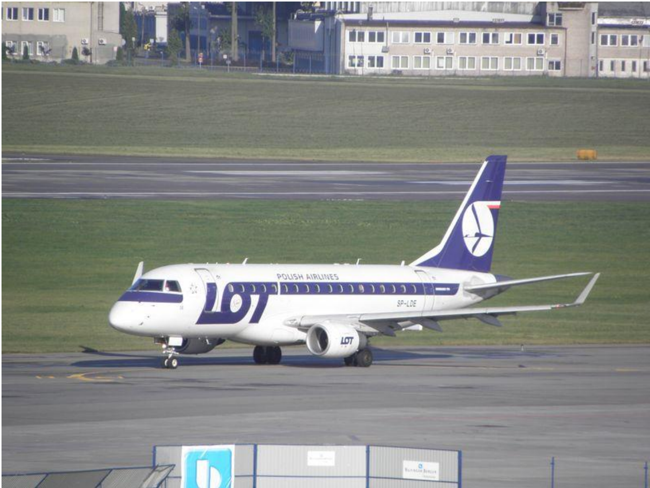
Figure 5. The most ubiquitous code C aircraft provide limited cargo capacity. Embraer 170 can carry about 1 tonne of cargo or less (different airlines offer various capacities).
